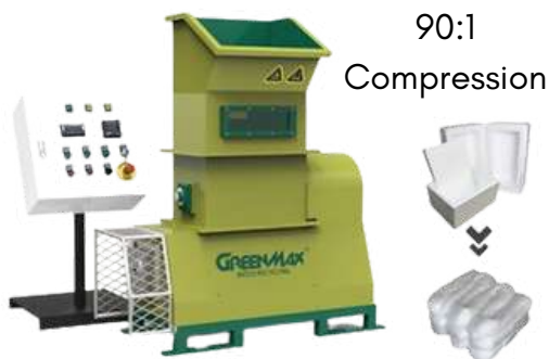
Figure 25: Hot melt compactor
