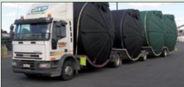
RX Plastics had the deck of a truck completely modified to be able to handle the transportation of their water tanks. They have maximised loading potential and ensured their product gets delivered safely and securely.
