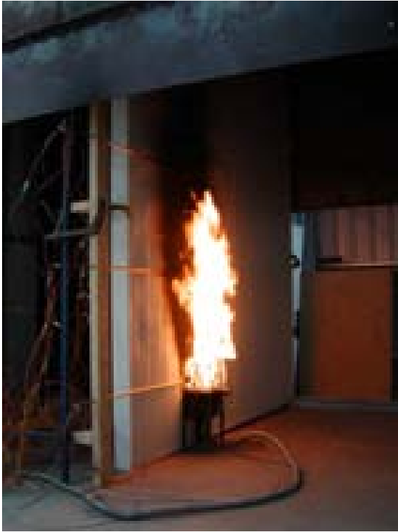
Figure 4.9: Trial 2 after 10 minutes at 100 kW.
