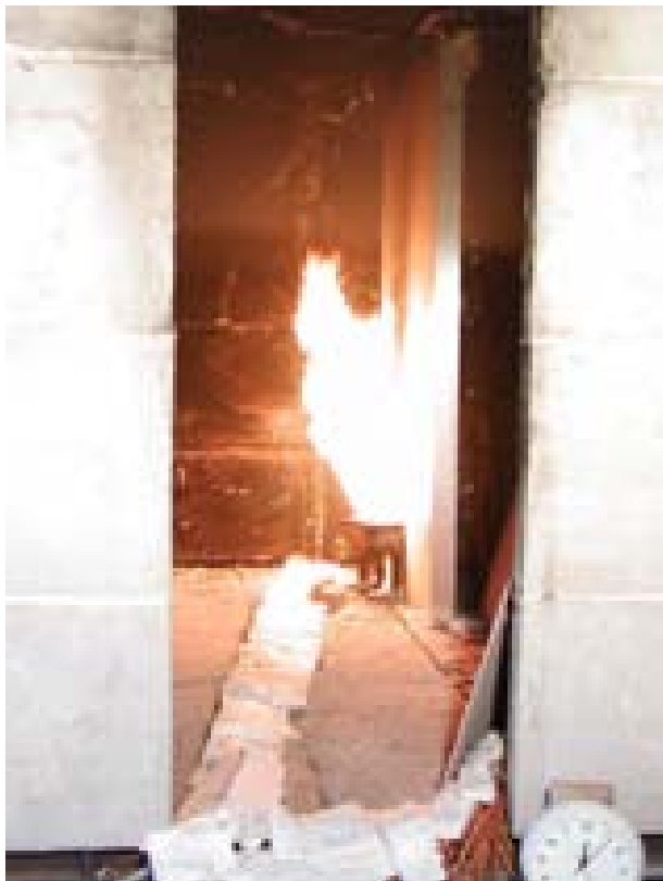
Figure 4.36: ISO9705 Room and joint 1 panel.
