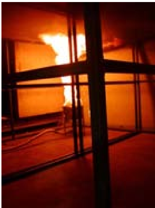
Figure 4.18: Trial 3 at 2 minutes and 100 kW.
